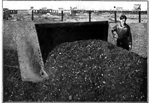
FIG. 5 THE SCRAPER HANDLES 60 TONS OF COAL PER HOUR
